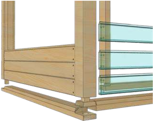
POST AND BEAM SYSTEM
