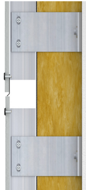
Raccord des profilés supports = joint des panneaux
